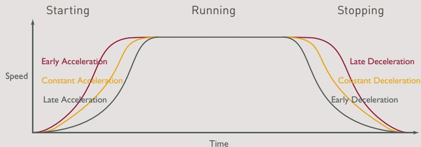
Adaptive acceleration offers three start and stop profiles according to your needs
