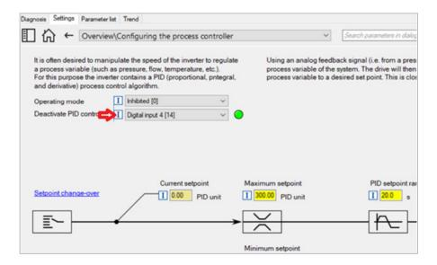
Next, set "Activate preset (bit 0) (P400:018)" to be triggered by the same Digital Input to trigger the purge (i.e. "DI4 [14]"). Finally, set the Purge speed (i.e. 60Hz) in "Preset 1 (P450:001)."
