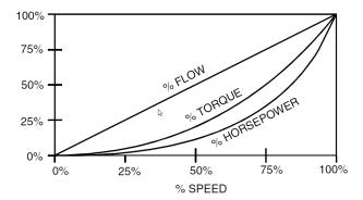
To do this, i500 drives can use a quadratic V/Hz profile to reduce the voltage supplied to the motor as a function of speed following the curve defined by the affinity law (following the torque curve). Dampers are another common flow control method. Compared to a damper, the lower power requirements of the i500 VFD provide a greater energy savings. Following the affinity laws. operating at 75% flow reduces power demand by over 50% with an i500 drive.
