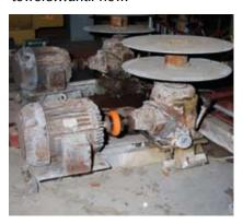
A "typical" cooling tower fan drive featured a right angle gearbox mounted under the fan powered by a driveshaft attached to an induction motor.
