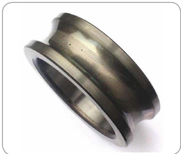
Figure 8: Fluting on the inner ring raceway of a bearing
