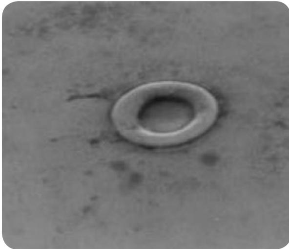
Figure 5: micro crater of a few um in diameter
