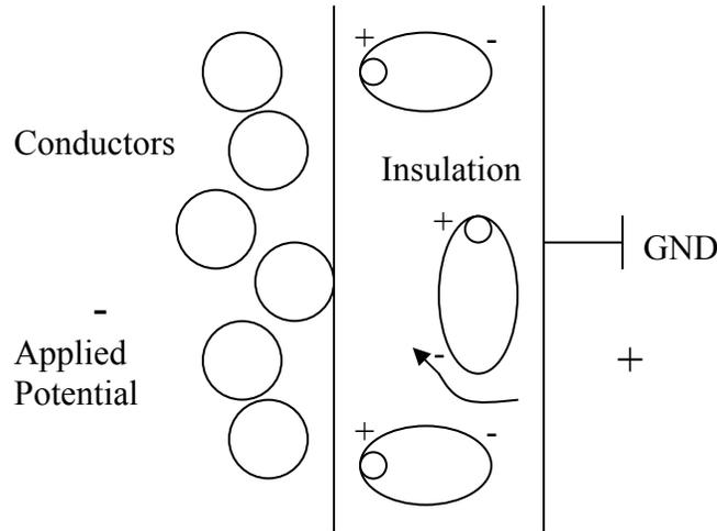
As current passes through conductors near electrical insulation, the insulation reacts by polarizing the atoms (dipoles) within the insulation. As the dipoles line up, there is less leakage (capacitance) between the conductors and ground. This also occurs in the insulation system between conductors when there is a difference of potential. In a good insulation system, the polarization of the insulation happens quickly. Once the potential is removed, the dipoles oppose each other and randomize.
