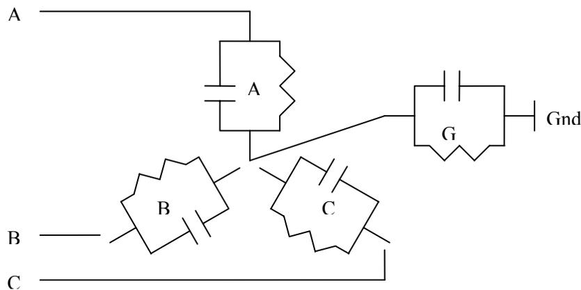
The electrical insulation circuit is modeled as a series of RC circuits between conductors and conductors and conductors and ground. As changes occur to the insulation system, the values of R and C change. The values of A, B, C, in Figure 2, are the sum of the turn to turn and coil to coil RC values of each phase. G is the sum of the insulation between the windings and ground for the complete circuit.
