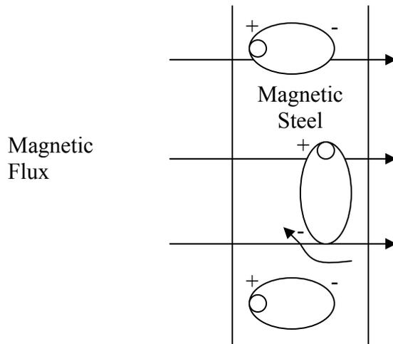
The same effect occurs in a magnetic field. The magnetic dipoles of the backiron and teeth of the stator core line up in the direction of the magnetic field. This helps direct the magnetic flux and adds to the strength of the fields within the airgap. The reluctance of the steel to change polarity shows up as hysteresis losses from the steel. Once the field is removed, the magnetic dipoles of the steel quickly randomize.
