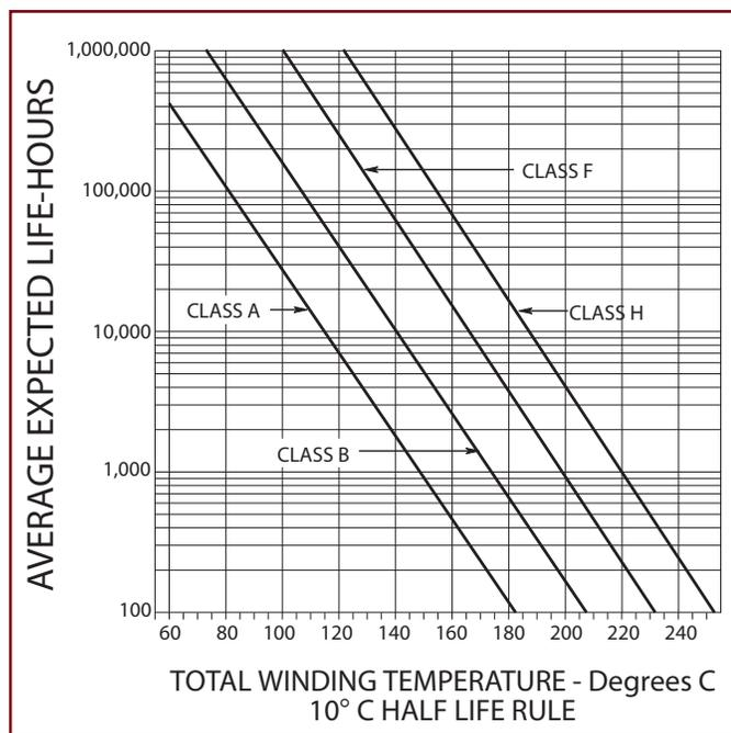
Figure 2. Insulation life vs. temperature.
