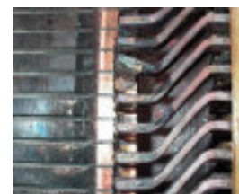
Broken commutator lead
