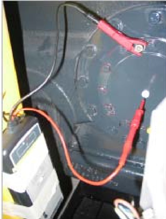
Opening for measuring sensor in the bearing cover
