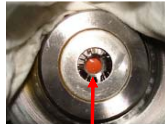
Opening for measuring sensor in the bearing cover
