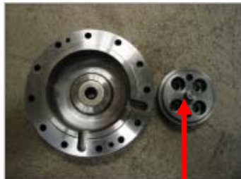
Opening for measuring sensor in the bearing cover
